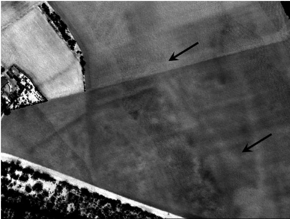
Fig 7 Lidar tile over Savernake forest showing the Roman road appearing as a feature due to the difference of the intensity of the returned signal (lidar © Forestry Commission; source, Cambridge University ULM (May 2006)).
