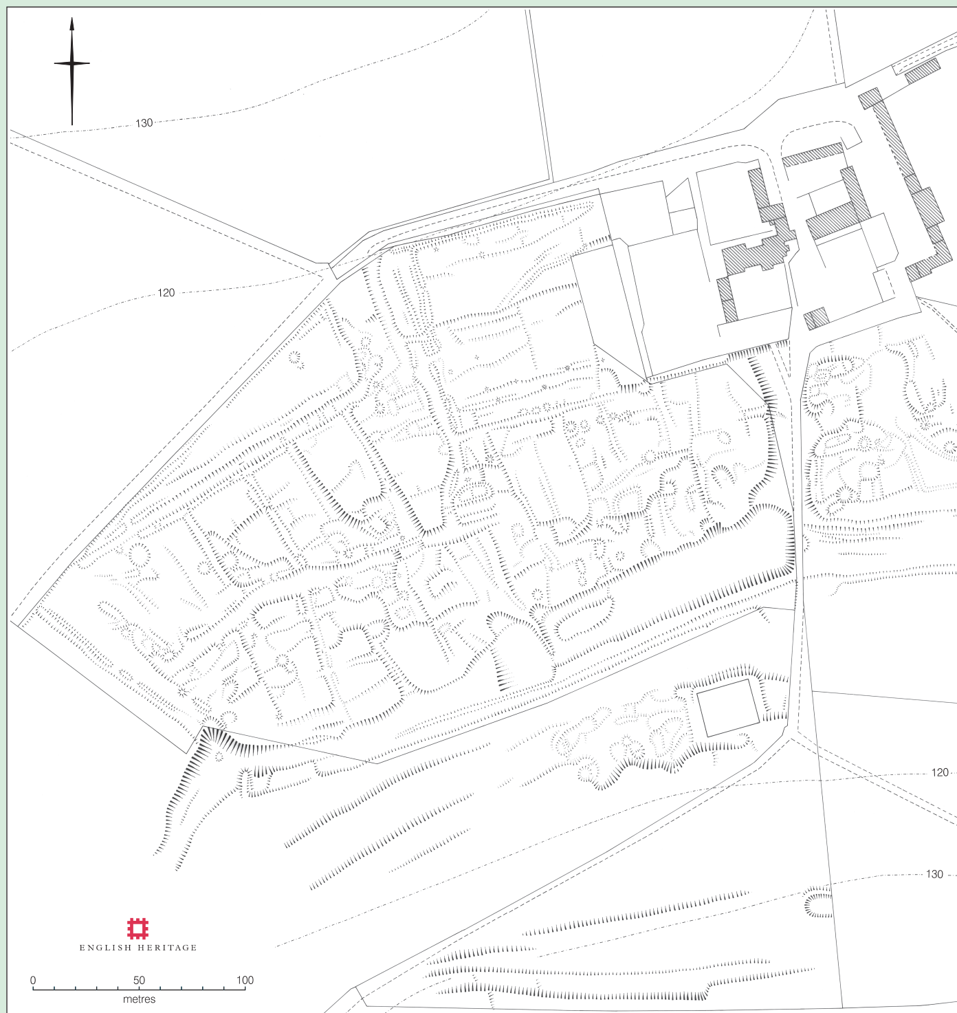
Earthwork survey of a deserted medieval village at Norrington in Wiltshire. This has been drawn using traditional pen and ink techniques and is reduced from the original 1:1 000 scale survey.
