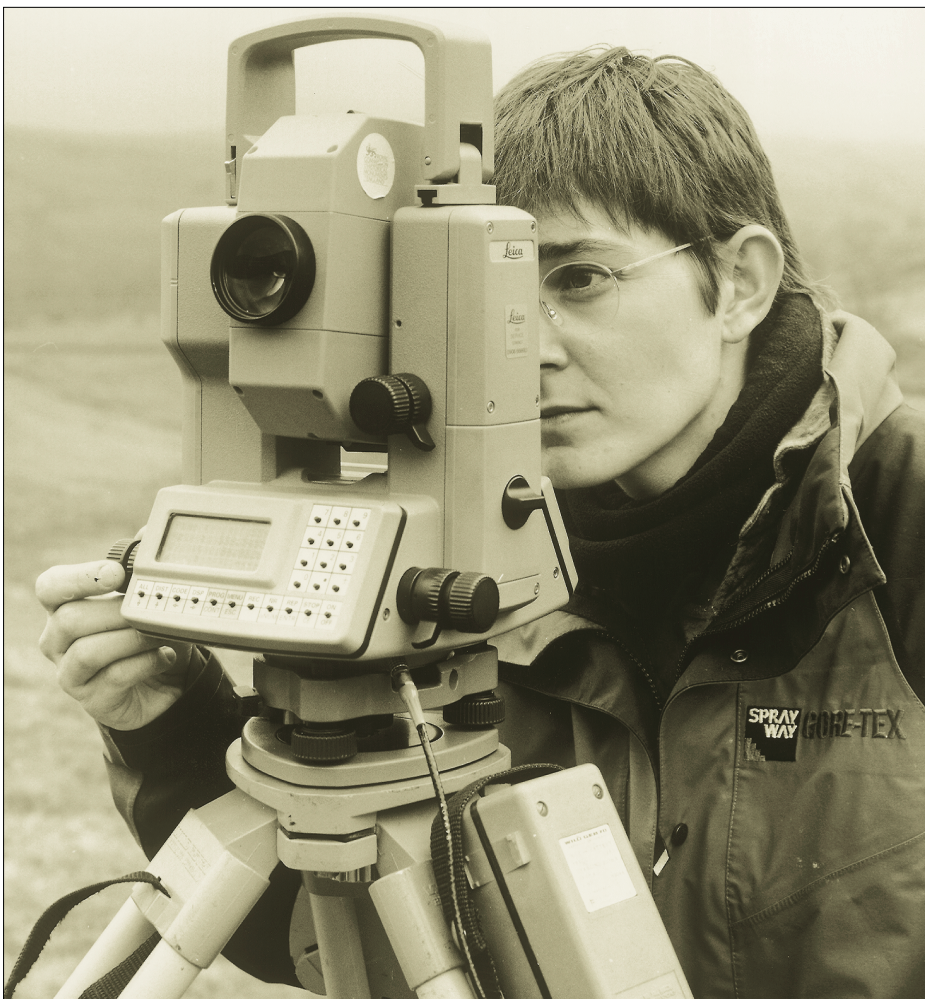
Figure 2 'Total station' EDM: electronic survey instruments supply control to a high degree or accuracy, but are not absolutely necessary for archaeological survey. Indeed, it is worth remembering that before the 1970s all survey was done without benefit of electronic instrumentation, to levels of accuracy far higher than those needed for archaeological earthwork survey.
