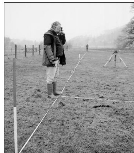
Figure 4 The optical square in use, raising a long offset from a tape line.
