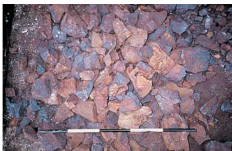
Figure 8 Roasted and crushed iron ore, prepared for smelting experiments. (Photograph by Peter Crew). Iron ores vary in colour and can be difficult to spot, particularly if they have not been roasted, as they do not necessarily have a strong colour or high density. Roasted ores (see photograph) are commonly red, purple or orange, because they are oxidised. Ore fines are small particles of roasted ore that sometimes respond to a magnet and have high magnetic susceptibility. Pieces of reduced ore, sometimes partially slagged, are sometimes found among the debris from the bottom of the furnace, and these are commonly grey. The minerals present in iron ores can be determined using X-ray diffraction, and the iron content can be determined by chemical analysis (p 25). The ores recovered during archaeological fieldwork need not be representative of the ores smelted because, for example, they might have been discarded because they were of poor quality.
