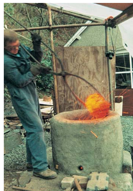
Figure 1 Experimental iron working at Plas Tan y Bwlch: removing an un-consolidated bloom from a furnace. (Photograph by David Starley)
