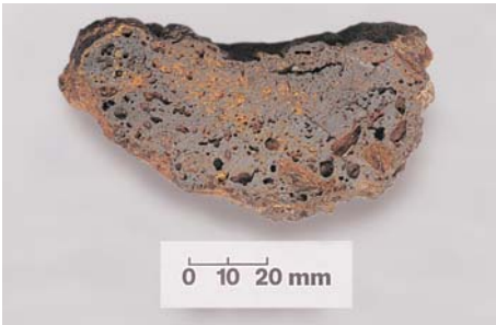
Figure 21 Cross section of a smithing hearth bottom. These are normally plano-convex to concavo-convex in section and circular or oval in plan. Their size and weight can vary considerably, from 100g to more than 2kg, although the majority weigh 200–500g. The upper surface sometimes has a depression produced by the air blast, or is sometimes irregular, where the last formed slags have not been fully incorporated. The lower surface usually has impressions from charcoal or the hearth lining. The size of the cake depends on the amount of iron forged, how much slag it contained, whether fluxes were used and how often the hearth was cleaned out. The larger smithing hearth cakes can easily be misinterpreted as furnace bottoms. Smithing hearth bottoms from primary smithing, or refining will generally be larger than those from secondary smithing. Smithing hearth bottoms are sometimes slightly magnetic as they can contain fragments of iron broken from the bloom and some hammerscale.
