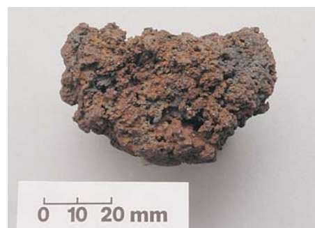
Figure 11 Iron blooms are rare finds on archaeological sites: here an ethnographic example is shown. Blooms are made up of many small particles of iron coalesced into a spongy lump. They are often badly corroded and fragmentary and are strongly magnetic.
