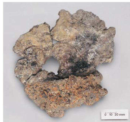
Figure 10 Vitrified clay lining with a blowing hole, from the Roman site at Ribchester, Lancashire. Note the slag attached below the blowing hole. Vitrified furnace lining is produced by a high temperature reaction between the clay lining of the furnace and the alkaline fuel ashes or slag. The outer parts are usually orange (oxidised-fired) ceramic, while the inner zone is grey or black (reduced-fired) and often vesicular with a glassy surface. Furnace linings might have been repaired repeatedly or replaced, and can show a sequence of vitrified layers. Although furnace walls were relatively thick, usually only the inner surface survives, or is noticed, as the heat of the furnace will not have fired the outer part. The hottest area of the furnace was near the blowing hole (see photograph), and consequently vitrified clay lining containing the preserved outline of the hole is often recovered. From the Roman and medieval periods there is some evidence for the use of replaceable circular or rectangular blocks of clay, with a blowing hole, that could be set in place in a prepared cavity in the furnace wall. These are often referred to as replaceable block tuyères.
