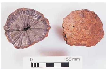
Figure 41 Pyrites nodule. The weathered outside (right) may look like iron slag but the interior (left) has a silver colour and radial structure.
