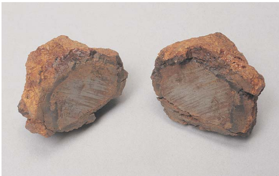
Figure 12 A consolidated iron billet from the Roman site at Westhawk Farm, Kent, that has been cut in half (max dimension 40mm). Partially consolidated billets are more common finds than blooms. They vary in size, are often badly corroded and fragmentary, and are strongly magnetic.
