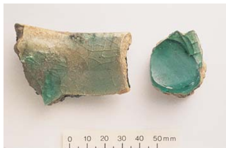
Figure 37 Ceramic crucible sherds with a thin layer of glass on the inner surface from Glastonbury, Somerset. Crucibles containing glass, dribbles of glass and lumps of glass cullet are all evidence for glass re-melting, which was commoner than glass making until the late medieval period.
