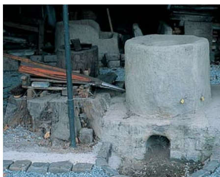
Figure 9 Bloomery furnace reconstruction (external diameter 0.7m). The tapping arch, through which the liquid slag enters the tapping pit, can be seen at the front of the furnace. See Figures 1 and 4. (Photograph by Sarah Paynter)
