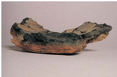
Figure 26 Part of the cope from a cauldron mould from Prudhoe Castle, Northumberland. Note the inner surface in reduced-fired (black) but the outer surface is oxidised-fired (red).
