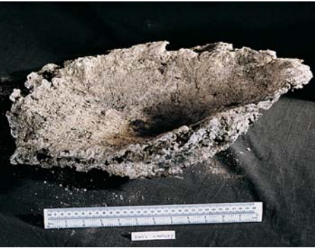
Figure 30 Lead melting dross that solidified in a hollow in the ground, from Kings Langley, Hertfordshire. It is a mixture of lead metal and oxides that were skimmed off the molten metal before it was cast.
