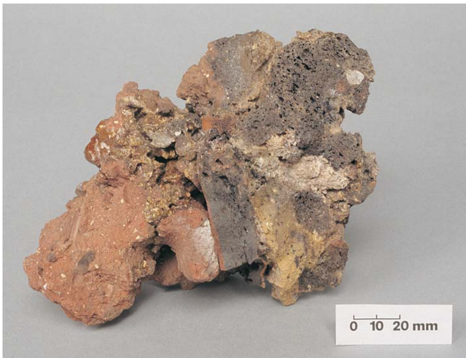
Figure 39 Daub and ceramic tiles from a Roman building in London destroyed by fire, which are stuck together by an accidentally-formed lead-rich glass.
