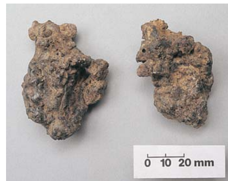
Figure 15 Undiagnostic slags (from Housesteads, Northumberland) are small or fractured pieces of slag that have the dark colour of iron-rich slags, but do not have any diagnostic surface morphology. Therefore, although indicative of iron-working, they cannot be used to distinguish between smithing and smelting. They are sometimes the largest proportion of slags in an assemblage.
