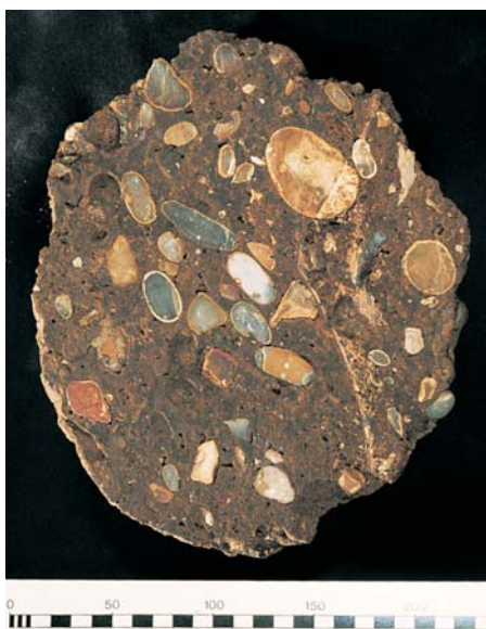
Figure 40 Section through a puddingstone boulder; the rounded exterior can be mistaken for iron slag.
