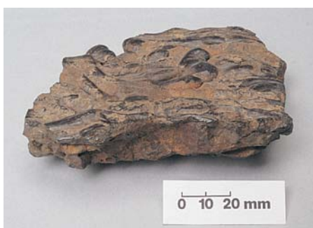
Figure 14 Tap slag has a characteristic shape, resembling a flow of lava, with rivulets of slag on the upper surface and a rough under surface which may have adhering sand or clay. Tap slag is dense with few relatively large bubbles, as it flows out while hot and fluid. It is dark in colour, usually grey to black, sometimes with a liverish or maroon upper surface. The size of tap slags can vary from individual runs of a few hundred grams to accumulations weighing 10kg or more. Hot, fluid slag can also form long, thin runs.
