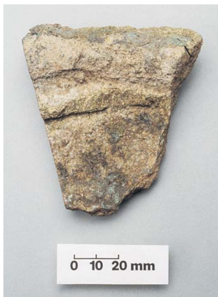
Figure 34 Segment of a litharge cake from Thetford, Norfolk. Examples up to 200mm in diameter and 30mm thick are known. They have a flat or convex base and normally have a central depression in their upper surface. They are very heavy for their size because of the lead in them and are fairly powdery and friable. Litharge cakes vary in colour from grey to greenish if much copper is present.
