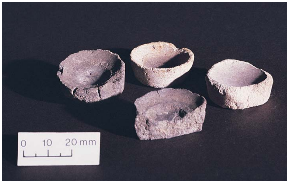
Figure 32 Bone ash cupels from the Tower of London. They are pale coloured and powdery. The absorbed lead in these objects makes them noticeably heavy for their size.
