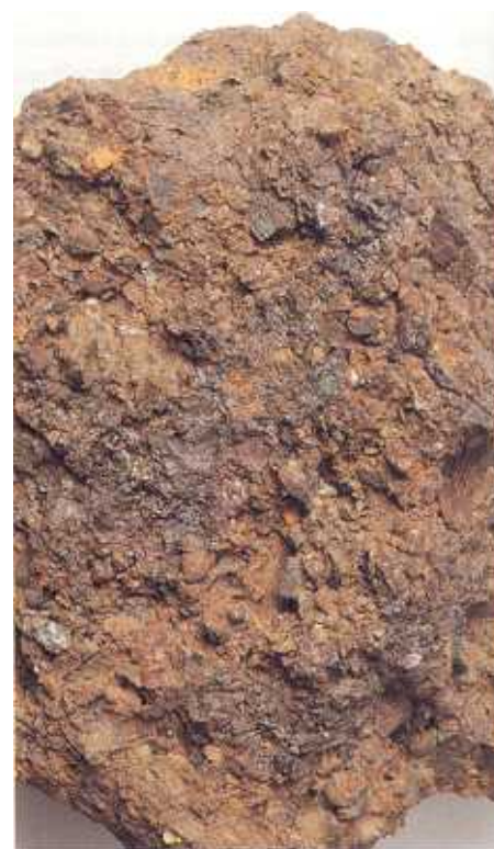
Figure 20 Smithing pan from the Roman site at Westhawk Farm, Kent. It consists of a layer of debris, largely hammerscale, trodden down and corroded together (image 100mm high).
