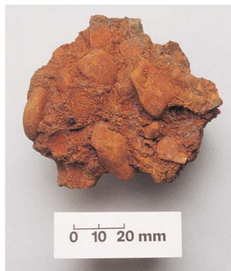
Figure 42 An iron concretion consisting of pebbles and sand grains bound together by iron compounds. They are amorphous orange-brown lumps that respond poorly to a magnet but do not have the typical vitrified surfaces of metal working debris. They form as a result of the re-deposition of iron compounds in a similar manner to the natural phenomenon of iron panning. The process is sometimes enhanced by the presence of iron objects or scrap metal.
