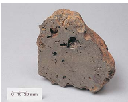
Figure 13 Section through an Anglo-Saxon furnace bottom from Mucking, Essex. Furnace bottoms are dense, dark-coloured slags that solidified in the furnace and can retain the shape of the furnace base, sometimes with part of the baked clay structure attached. Furnace bottoms are typically 0.3m in diameter and 0.2m high, and will often contain pieces of reduced ore and fuel.
