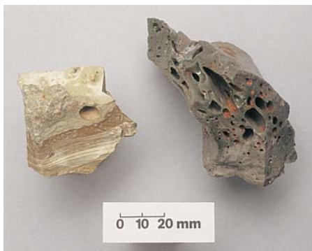
Figure 16 Blast-furnace slags are usually glassy in appearance and range in colour from blue and green to grey or brown. They usually have abundant fracture surfaces with little or none of the original surface remaining. They are less dense than bloomery-furnace fayalite slags, as they contain much less iron. They do contain a small percentage of iron however, which gives them their colour. These slags can be found in large quantities and were often reused, for example as hardcore or scattered across fields to improve soil quality.
