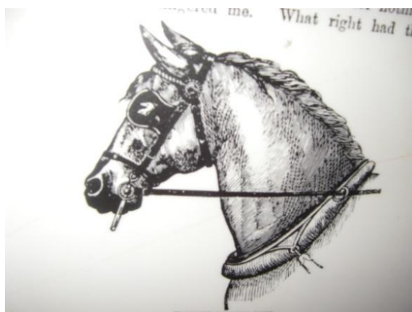
Fig. 12.30 Diagram of a hames in position on the collar © Bradford Industrial Museum
