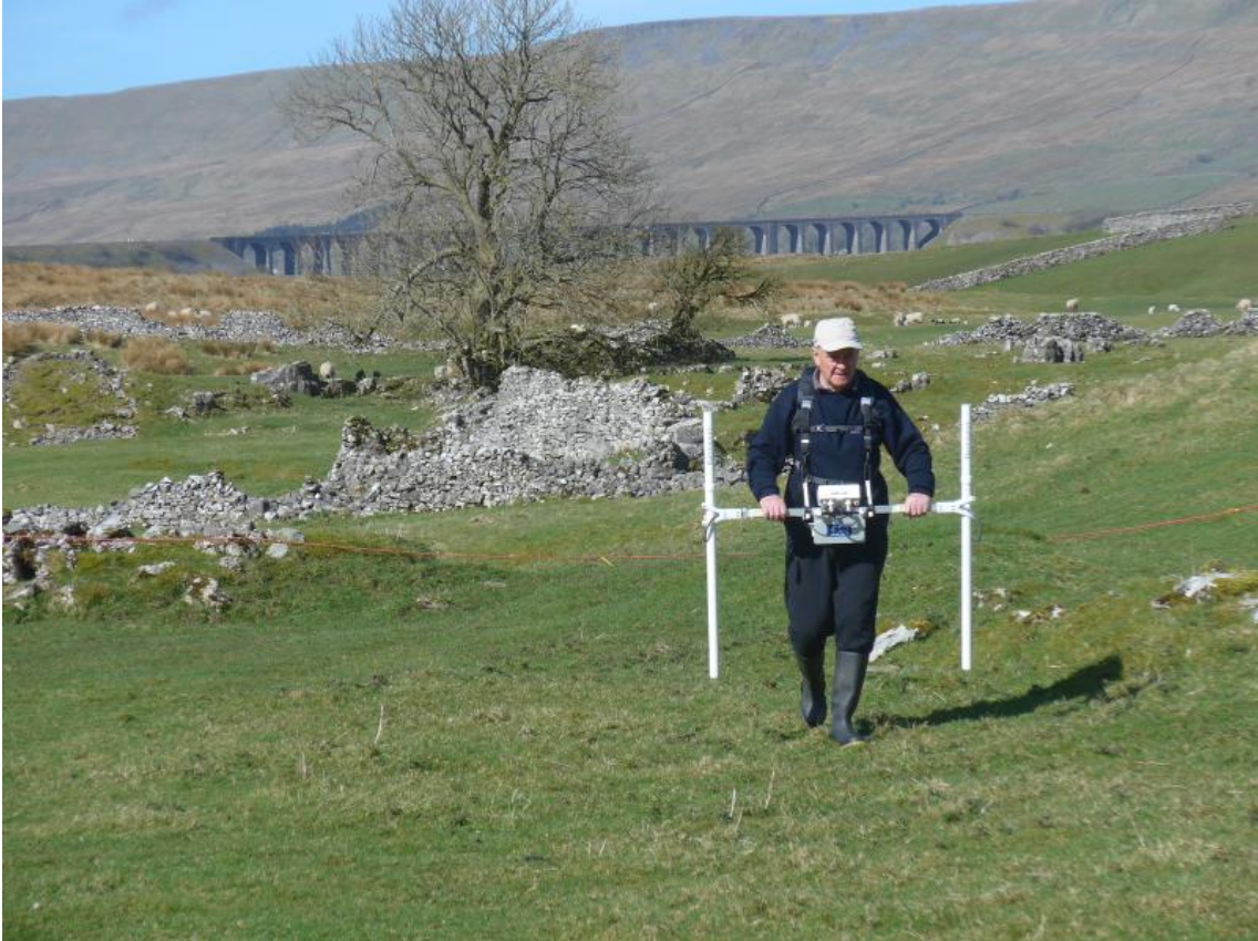
Fig. 11.1 Bartington gradiometer operated by SWAAG volunteer Mike Keenan (SWAAG)
