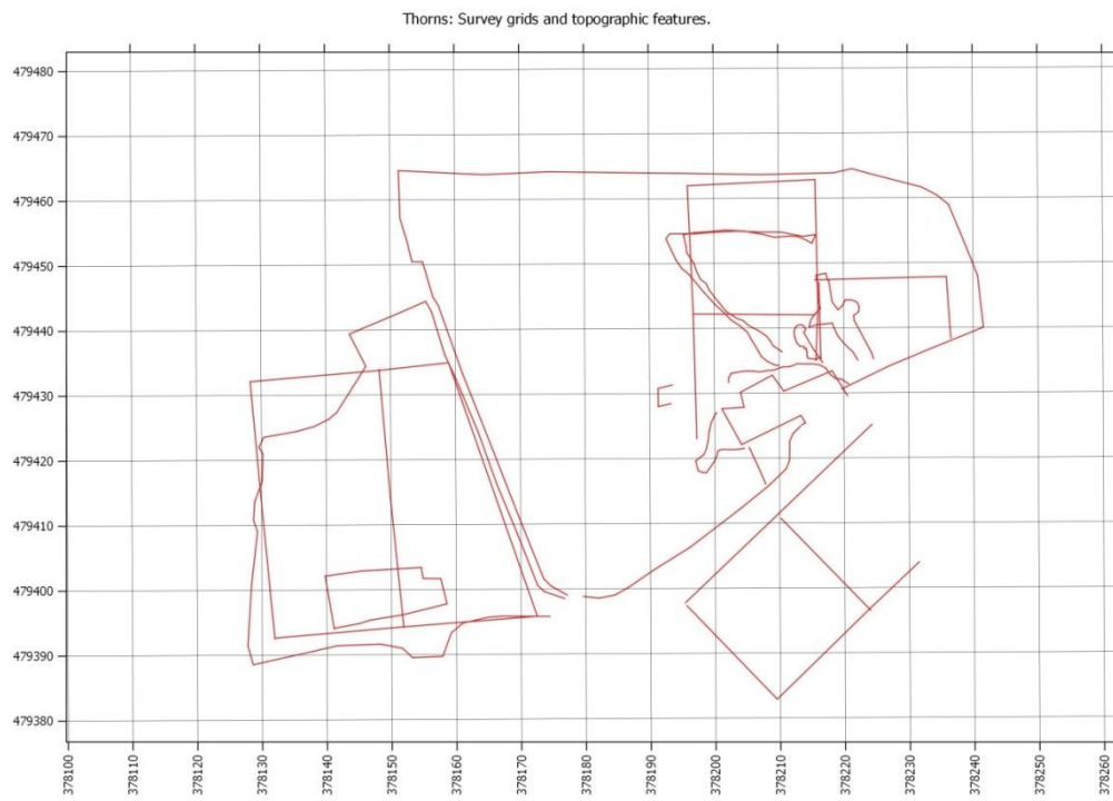
Fig. 11.14 GNSS data with survey grids and superimposed OS grid
