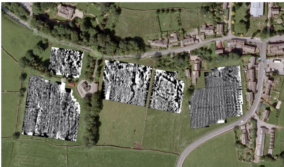
The results of the Grinton magnetometry survey overlaid on Google Earth.
