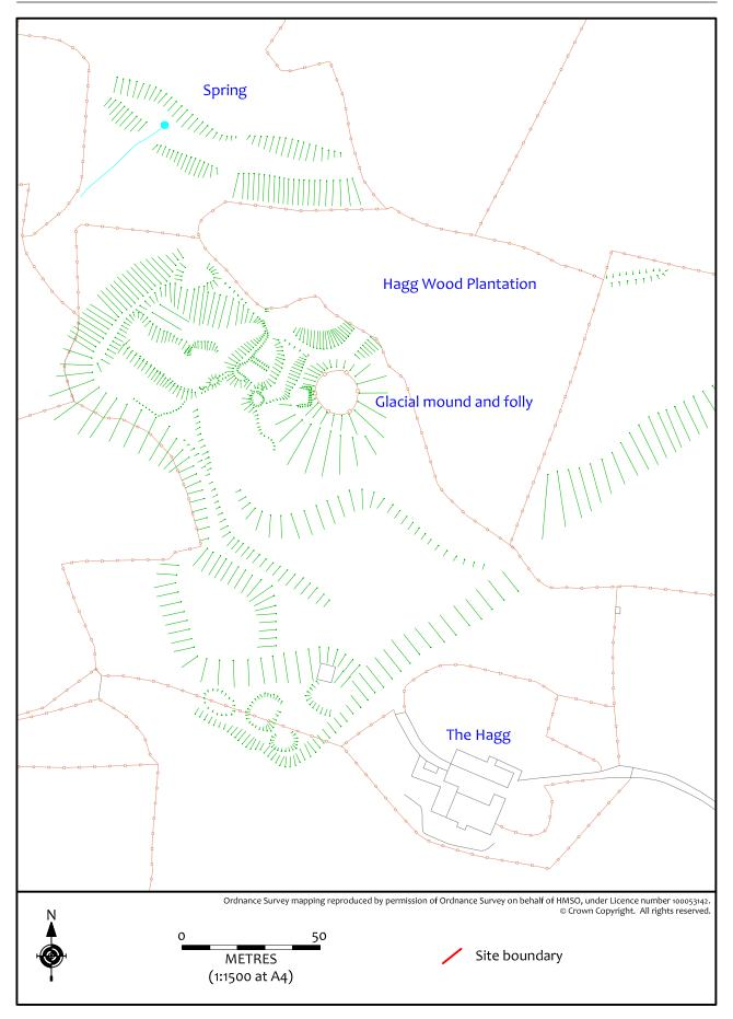
Figure 4. The results of the 2012 Total Station earthwork survey
