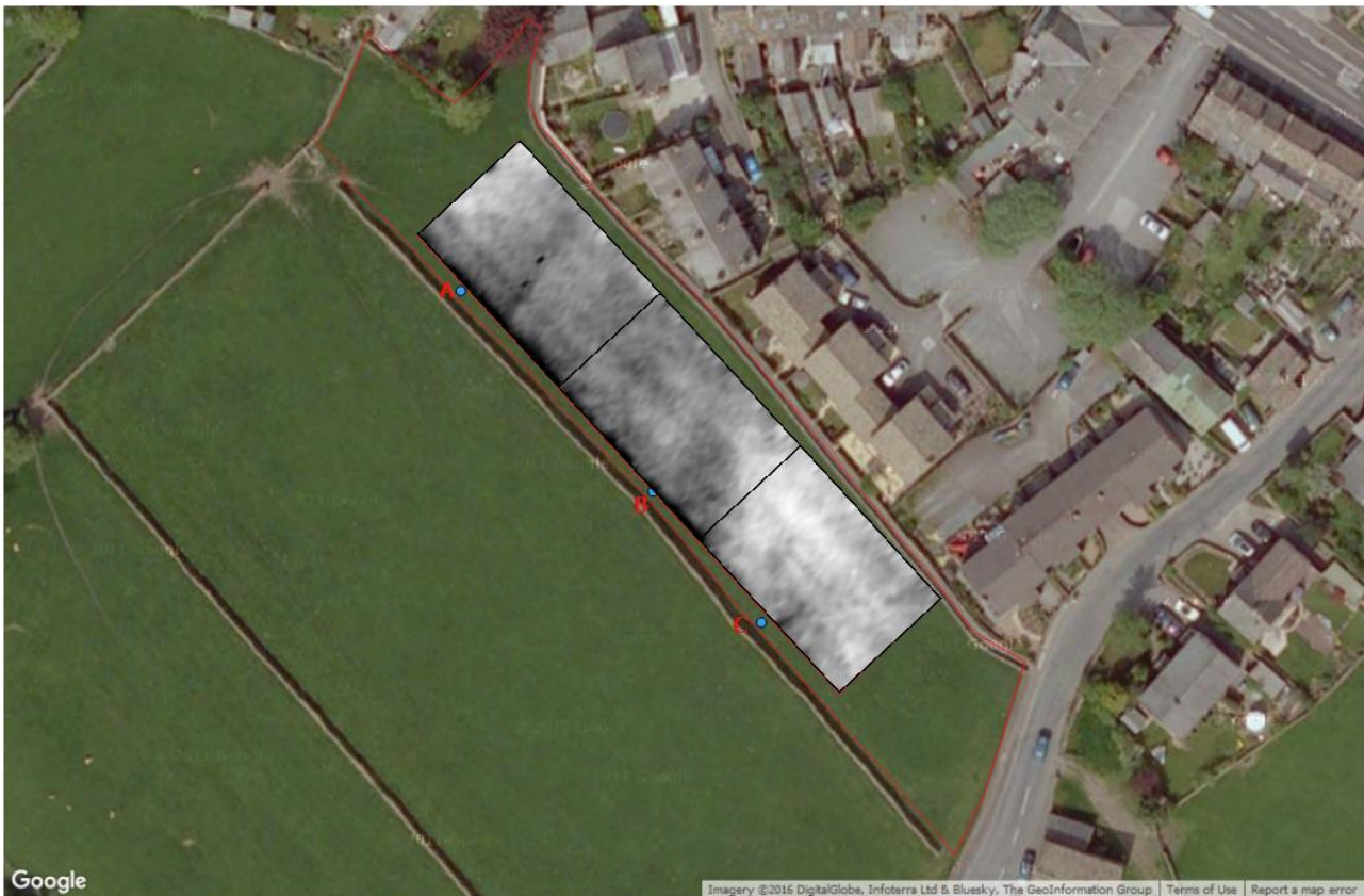
Figure 14: Site 2, Processed Resistance Survey data superimposed over Google Satellite image. (Clipped at +/- 2SD)
