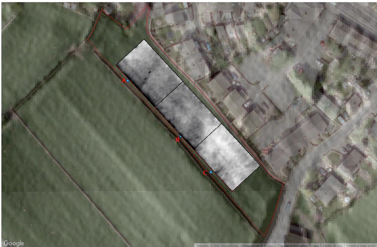
Figure 15: Site 2, Processed Resistance Survey data superimposed over LIDAR at 50% transparency over Google Satellite image. (Clipped at +/- 2SD)
