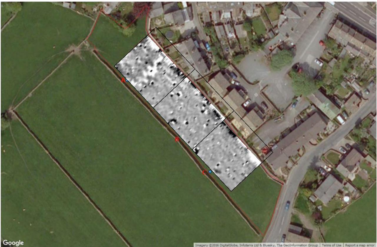
Figure 11: Site 2, Magnetic Survey data superimposed over Google Satellite image (Range -5nT to +10nT)
