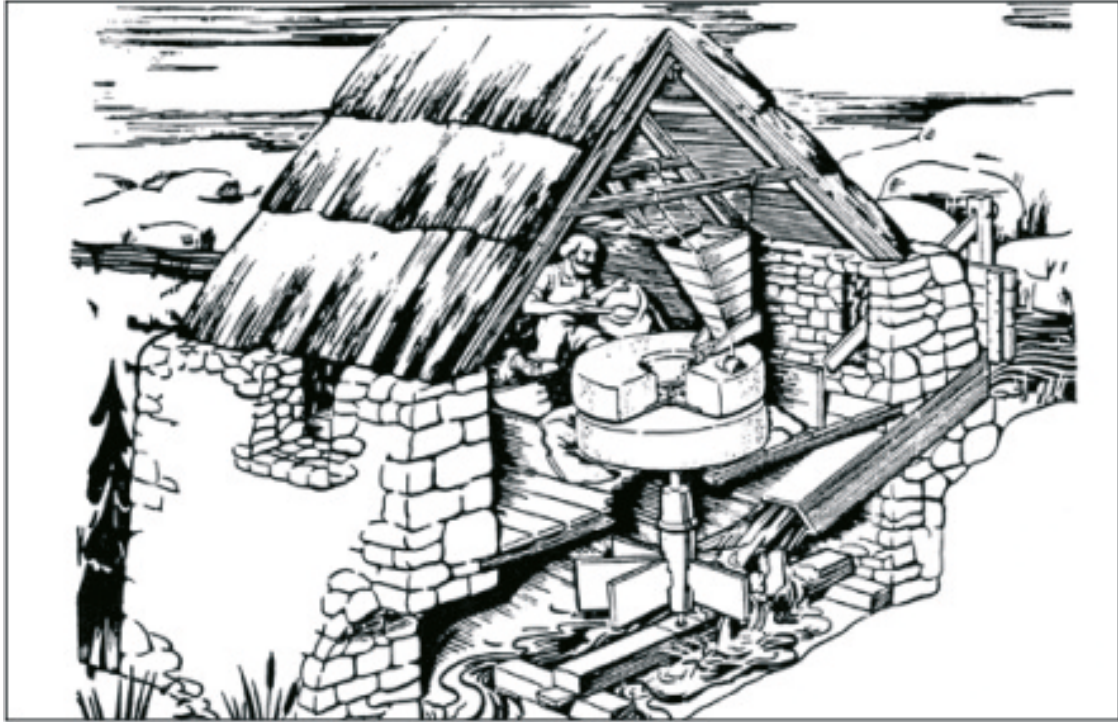
Image 16: English Heritage Introductions to Heritage Assets: Mills. Horizontal mill reconstruction based on a post-medieval example from Lewis, Hebrides.
